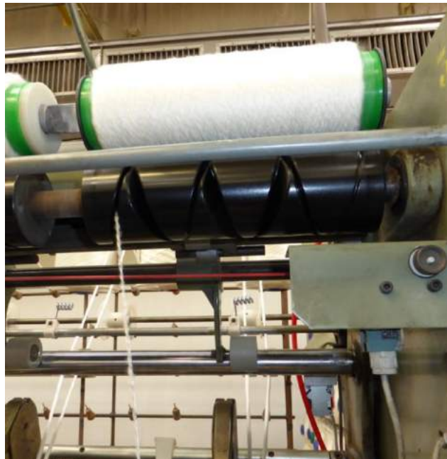
Figure 26: Storage unit placed above the wrap spinning system
